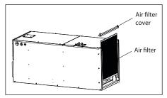
Fig. 4 — Remove the air filter cover
