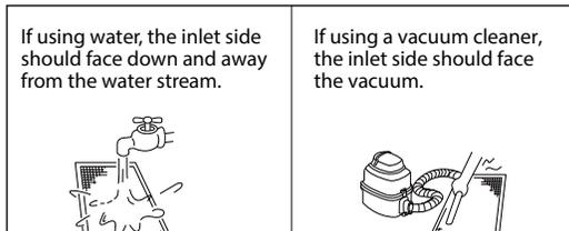
**Fig. 5 — Cleaning filter with water or vacuum**
