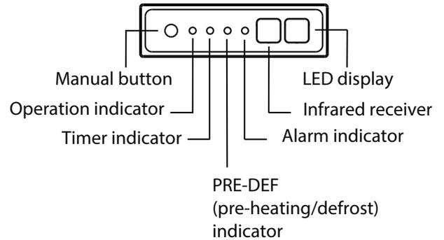
**Fig. 2 — IR (Infrared) Receiver Display Panel**
