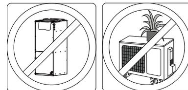
**Fig. 12 — Remove obstacles blocking air inlets/ outlets**
