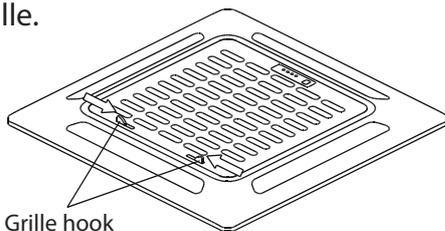
2. Hold the grille at a 45° angle, lift it up slightly and detach it from the main body.
