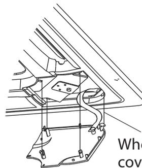
When installing the cover, slide the four slide fasteners into the corresponding slots on the panel.
