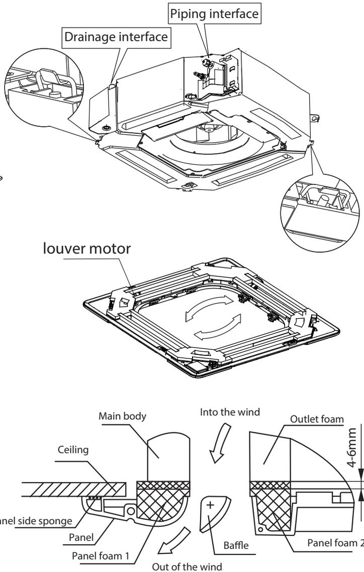
**NOTE:** If the height of the indoor unit needs to be adjusted, you can do so through the openings at the panel's four corners. Make sure that the internal wiring and drainpipe are not affected by this adjustment.
