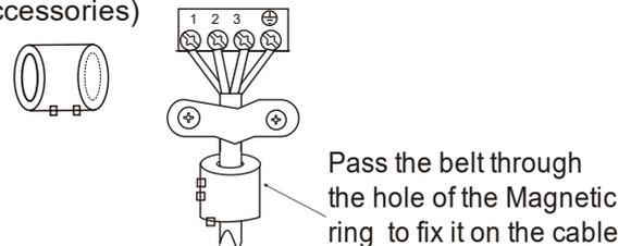
Pass the belt through the hole of the Magnetic ring to fix it on the cable
