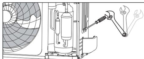
3. Connect the power cable and indoor & outdoor connection cable. Clamp down the cable with the cable clamp.
