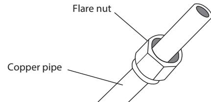
4. Remove PVC tape from ends of pipe when ready to perform flaring work.
