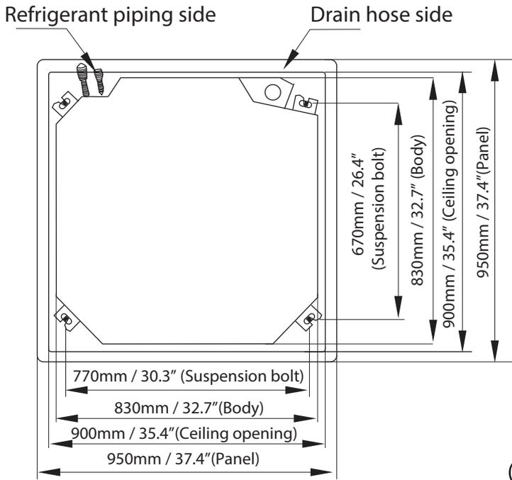
5. Mount the indoor unit. You will need two people to lift and secure it. Insert suspension bolts into the unit's hanging holes. Fasten them using the included washers and nuts.
