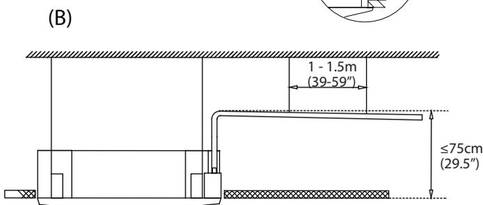
**NOTE:** When connecting multiple drainpipes, install the pipes as illustrated in the following figure.
