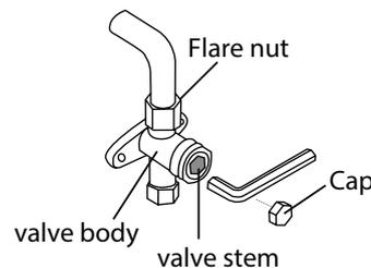
12. Using hexagonal wrench, fully open both the high pressure and low pressure valves.
