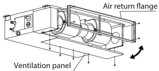
Bend the rear ventilation panel 90 degrees along the dotted line into a descending ventilation panel. (some models)
