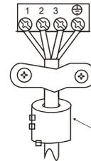
Pass the belt through the hole of the Magnetic ring to fix it on the cable
