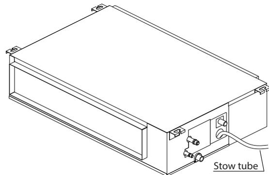
2. Turn on the unit in COOLING mode. You will hear the drain pump. Check whether the water is discharged properly (a 1-minute lag is possible, depending on the length of the drain pipe), Check whether water leaks from the joints.
