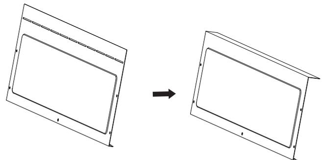
2. Change the mounting positions of the ventilation panel and air return flange.
