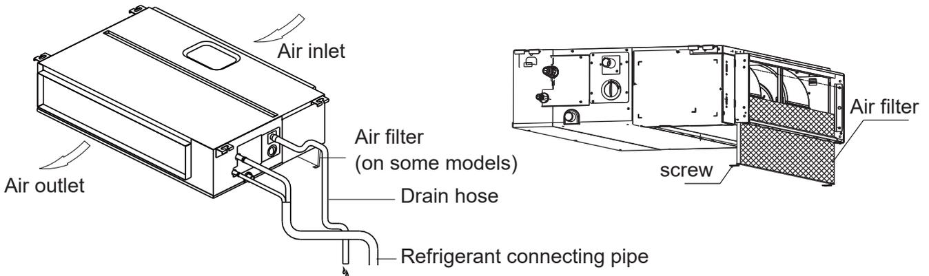
1. Put the filter into the flange subassembly through the bottom side;
