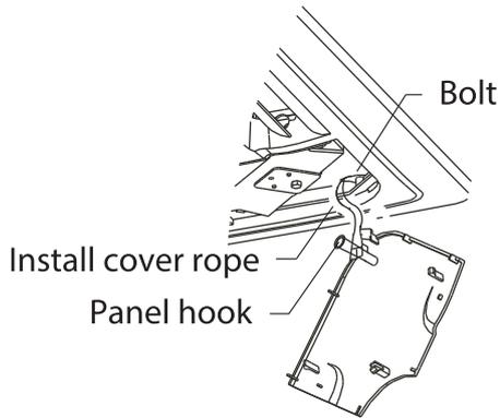
Re-installed into the style grid.
