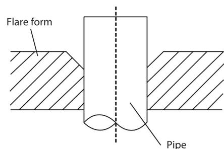
6. Place flaring tool onto the form.
