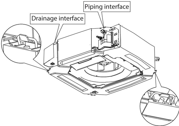
**NOTE:** If the height of the indoor unit needs to be adjusted, you can do so through the openings at the panel's four corners. Make sure that the internal wiring and drainpipe are not affected by this adjustment.
