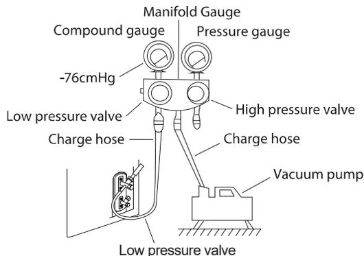
1. Connect the manifold gauge's charge hose to the service port on the outdoor unit's low pressure valve.
