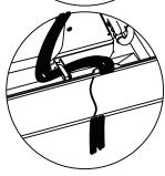
Replace foam gasket over wires.
