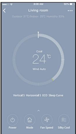
3.) Thus, the user can control air conditioners on/off status, operation mode, temperature, fan speed and so on.
