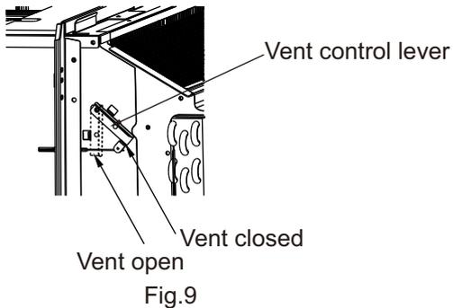
NOTE: When vent control lever set at CLOSE, only the air inside the room is circulated and filtered. When set at OPEN, some outdoor air will be drawn into room. This will reduce heating or cooling efficiency.
