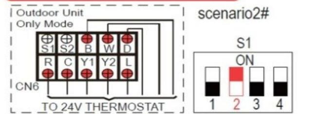
24V must never be connected to S1 – S2. All wiring must be in compliance with the above scenarios. Incorrect wiring will cause irreversible damage to control.
