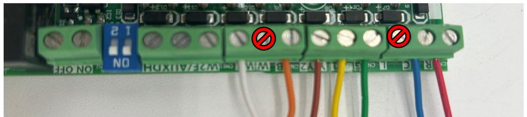
Up close view of 24 volt terminal strip on air handler. Please note which connections are used. Specifically please note that L & W are skipped.
